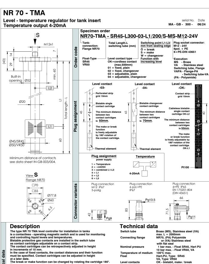
The break or make function can be changed by rotating the cartridge 180°. The permanent magnet fitted in the float switches the contacts if the level changes. The switching difference (hysterese) is 4 mm. For temperature monitoring,
